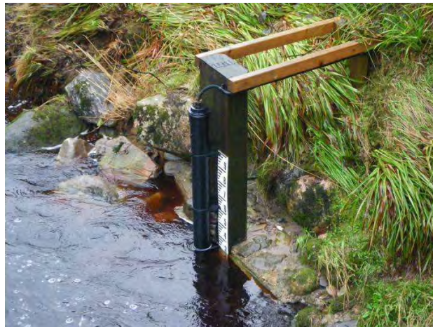
Figure 8: Example of temporary stage-discharge flow monitoring station
